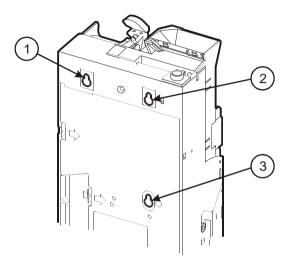
The vending machine is fitted with three screws in matching locations. Alternatively, there may be two location studs and one retaining screw, or a similar arrangement. Whatever the arrangement, there must be a retaining screw in the upper right-hand position.
