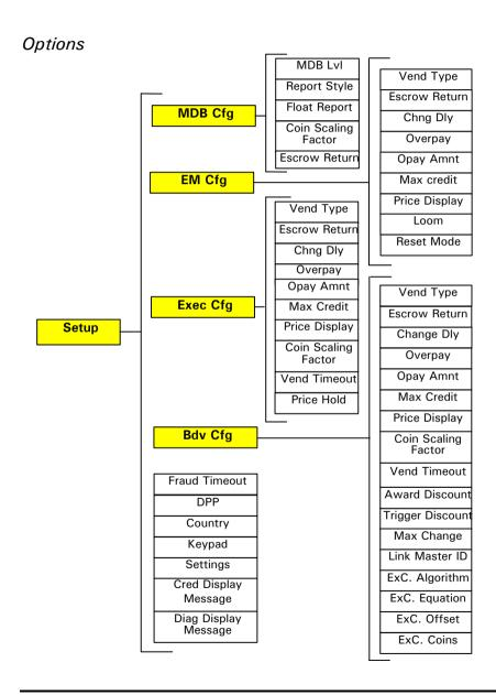
**Note:** Only one changegiver variant can be active at one time. The displayed message for the current variant includes the word 'Active', for example **MDB cfg: Active**
