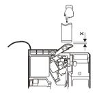
Check the alignment of the coin chutes. Insert two coins of each denomination into the vending machine and check that they cleanly enter the changegiver acceptor and exit from the changegiver into the coin return cup
