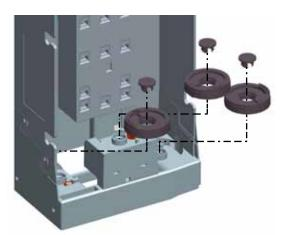
Fig. 5: Removing and reinstalling payout discs and lockings
