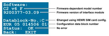
Fig. 17: Interface module diagnostics OK
