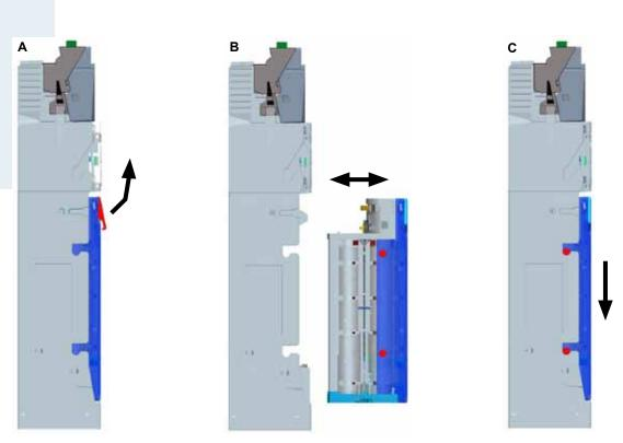
Fig. 1: Removing and reinstalling the coin cassette
