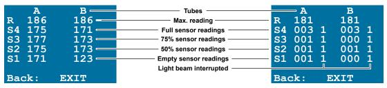
Fig. 8: Fine tube A&B readings with empty cassette
