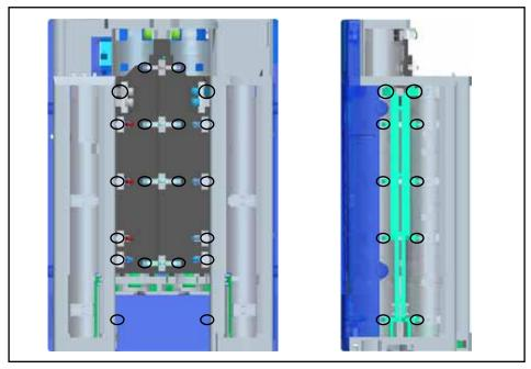
Fig. 10: Rear and side view of coin cassette all 45° surfaces accessible
