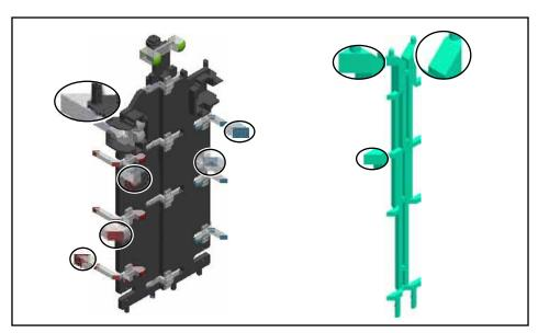
Fig. 13: 45° surfaces of light transmitter and light collectors
