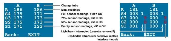
Fig. 24: Filling level sensor diagnostics OK
