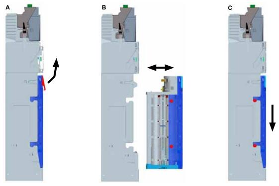
Fig. 4: Removing and reinstalling the coin cassette
